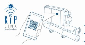
As an option, the direct control over the unit comes through the innovative **KIPlink interface**. Based on Wi-Fi technology, KIPlink gets rid of the standard keyboard and **allows one to operate on the unit directly from a mobile device** (smartphone, tablet, notebook).
